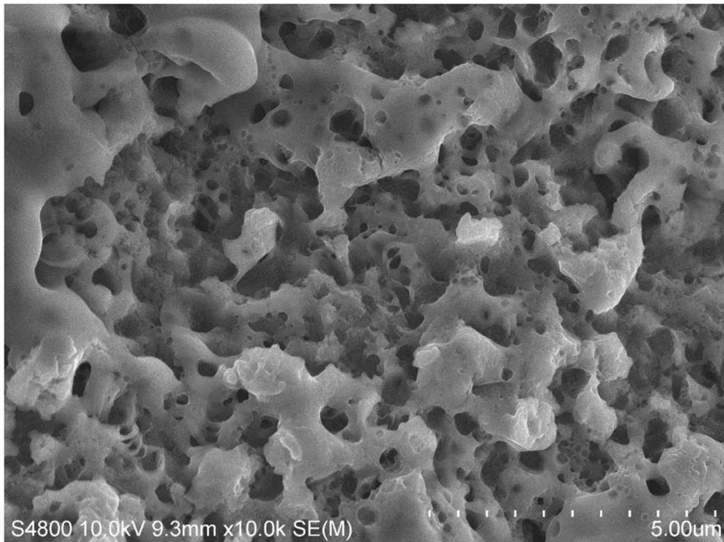
EDS and XPS analysis show a highly oxidated with a relative oxygen content increased by more than 30% versus a regular Sandblasted/Etched Titanium dental surface.
