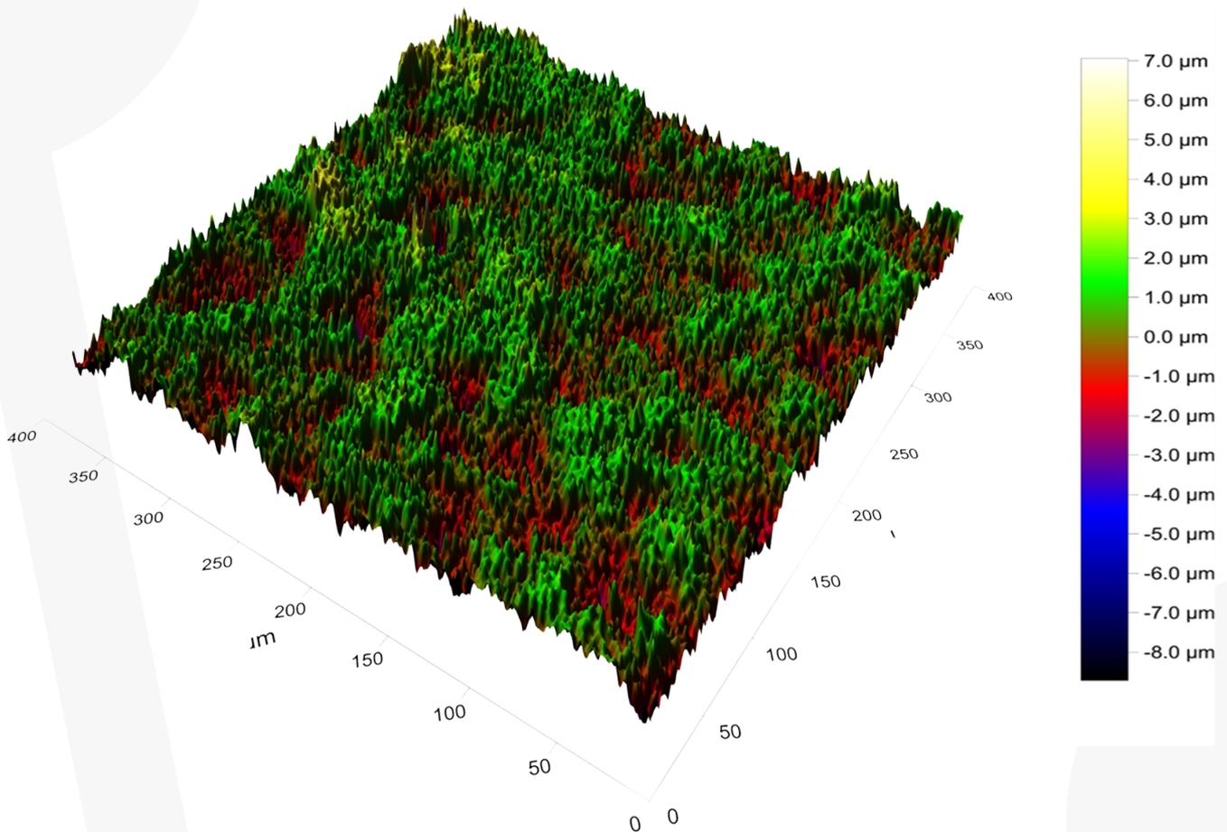
3D surface reconstruction and Surface roughness profile (R) was measured using a high-resolution, white light, non-contact laser profilometer (CyberSCAN CT 100, Cyber technologies, Eching-Dietersheim, Germany) with a z-resolution of 20 nm and a lateral resolution of 1 μm.
