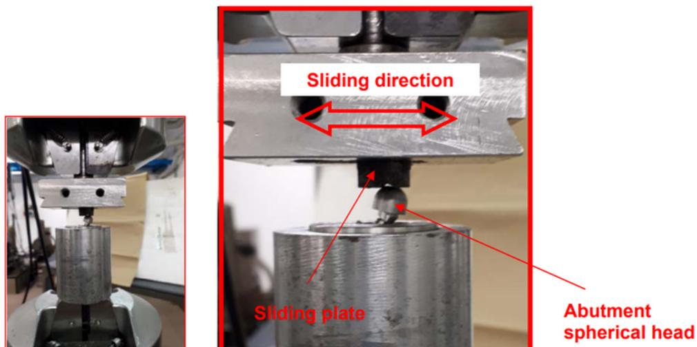
Figure 3 - Specimen during the test
