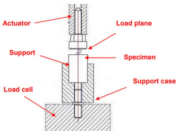
Figure 2 – Sketch of the experimental set-up for fatigue tests
