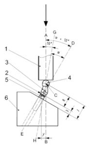
Figure 1. Implant configuration according to ISO 14801
